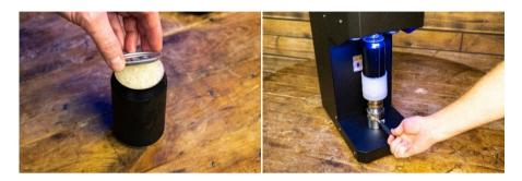
Place the can onto the spacer. Turn the seaming lever clockwise to raise the can until you feel soft resistance. Push through this resistance to lock the lever in position.
