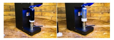
To seam 330ml cans, fit the 500ml can spacer and place the 330ml spacer adapter on top.
