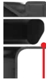
GASKET ORIENTATION Flat Side Into Lid Groove
