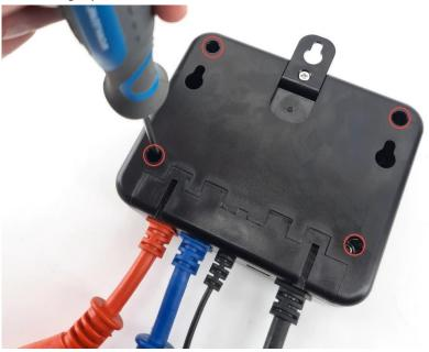
Unscrew the two screws which hold the slotted blanking plate to the housing and remove the slotted blanking plate.
